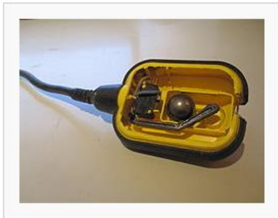
float switch on
