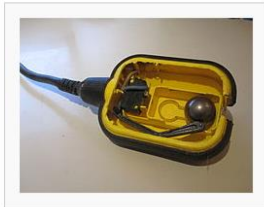
float switch off
